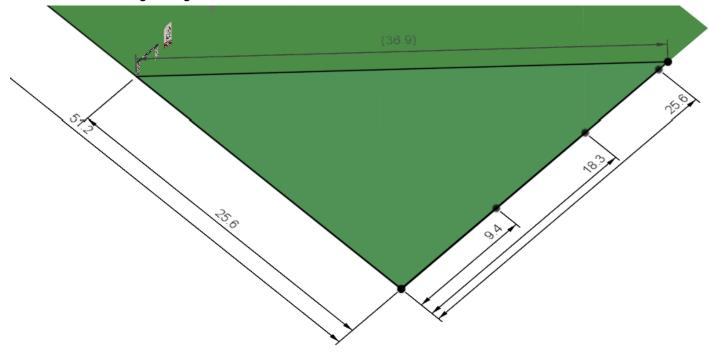
Step 4 We are now going to get the location for the 2 gates and flag. Take one tape measure and go to the 25.6m gate rebar and walk out 27.3m. Then with the other tape measure walk up 9.4m from the 51.2m mark. Where these 2 meet place a gate rebar.
