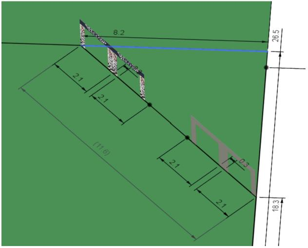
Step 10 We have one obstacle left, and by now you really love triangles or hate them! From the 26.5m mark walk out into the field 35.4m. Take the other tape measure and go to the 2 gates and flag you set up at the far end of the track. Place the tape measure on at the leg of the gate, NOT the flag, and then walk out 20.5 m. Where these 2 meet place a gate rebar for the gate. You can also place a rebar for the hurdle here. The hurdle rebar can be placed here, as well.
