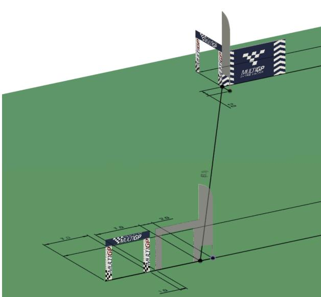
On the line from the 26.5m mark on the ground, walk back down the line 3m and place a rebar for the hurdle, 32.4m on the tape. Now to square the gate, walk 3.7m from the 32.4m mark for the hurdle out to meet the 2.1m line from the gate rebar you placed. Here is the last gate leg,
