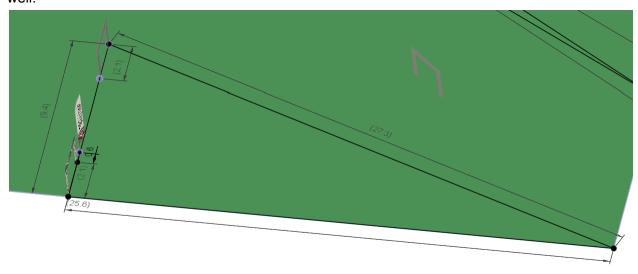
Step 8 From the 9.4m mark walk out 30.3m. Then from the 25.6m mark walk out 25,6m, where these meet place a flag stake. Now from the 9.4m mark walk out 17.9m and from the 18.3m mark walk out 15.5m. Where these meet, flag stake.
