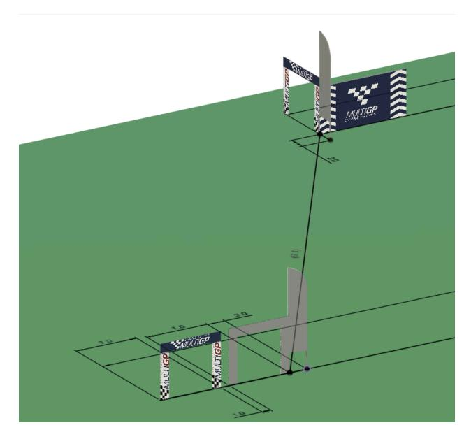
On the line from the 87 ft mark, walk back down the line 10 ft and place a rebar for the hurdle, 106 ft on the tape. Now to square the gate, walk 12.2 ft from the 106 ft mark for the hurdle out to meet the 7 ft line from the gate rebar you placed. Here is the last gate leg, place a rebar. If you are going to place a feather flag, place it 2 ft from the gate. You may also use a flag on the gate for this obstacle. When done it should look like this.
